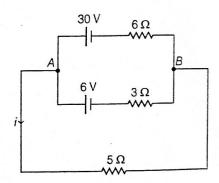
Using Kirchhoff's rules, we can find current (i) and potential across each cell as by assuming current in different part as shown
